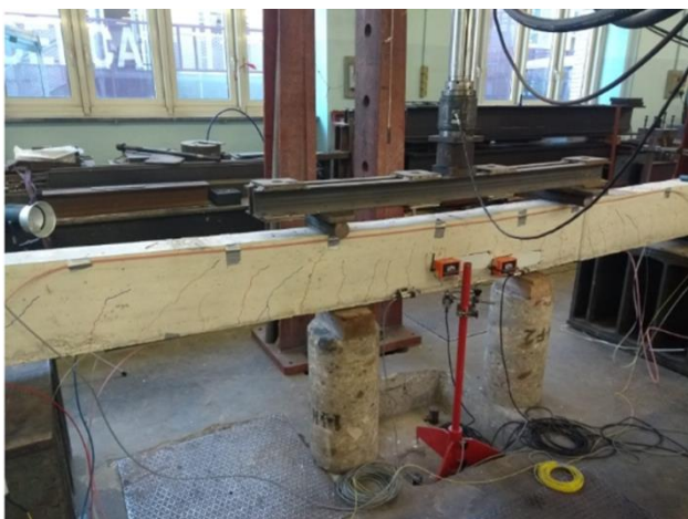
Figure 7. Cracks on tested beam.
