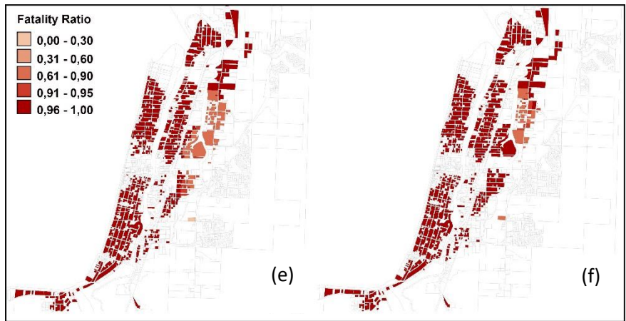
Figure 5. Fatalities for each building in good (a, b), fair (c, d) and poor (e, f) ambient condition. Tsunami-only scenario (left - a,c,e). Earthquake & tsunami scenario (right - b,d,f).
