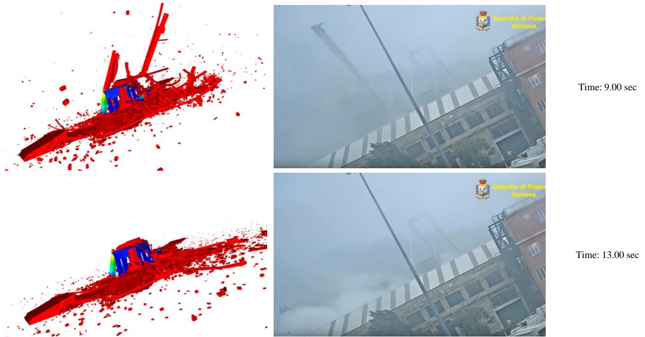
Fig. 18 – Side by side comparison of the collapse mechanism of the bridge. Analysis results (left), actual collapse images (right) [9].
