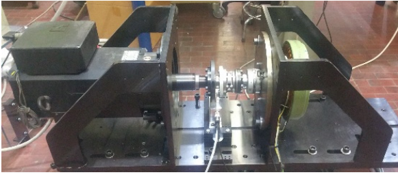
Fig. 9. View of the machine under test (right) and the driving machine (left).
