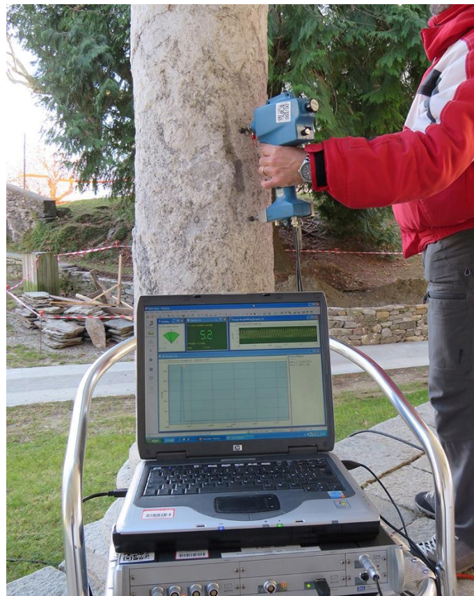
Figure 5. Setup of the impact test.
