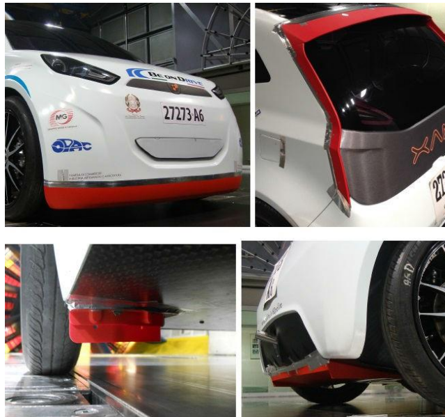
Fig. 7. Aerodynamic features (from left to right: bumper, spoiler and finlets, lokari dams, diffuser) mounted on the vehicle in wind tunnel test
