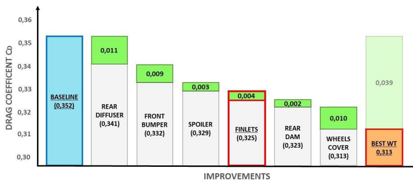
Fig. 8. Wind Tunnel best results at 70 km/h
