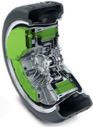
Figure 1 - Schaeffler's E-Wheel drive [11]
