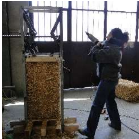
Figure 13. Pre-stressed straw bale.
