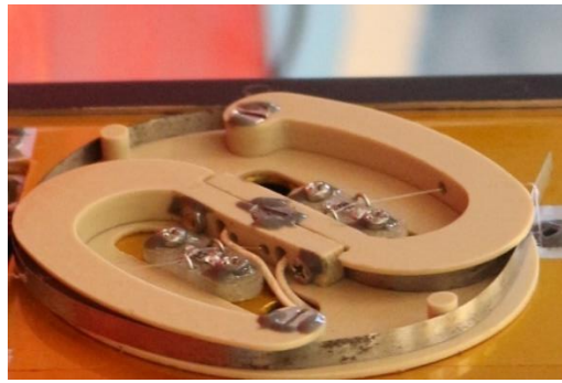
Figure 8. Antenna deployment mechanism with the antenna folded around.
