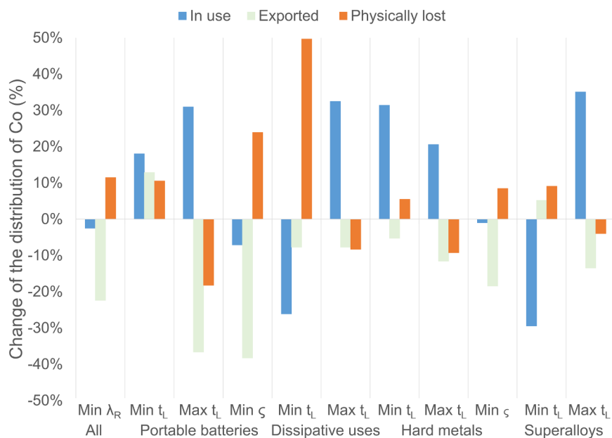
Fig. 3. Effect of 11 parameters (per application) on the distribution of Co: in use, exported, and physically lost, when they take their minimum or maximum value. The results present the average of the annual change from 2015 to 2040, in comparison to the baseline scenario (BAU). Min: minimum value of the parameter, Max: maximum value of the parameter, All: all product categories, \lambda_R : recycling efficiency, t_L : lifetime, \zeta : collection-to-recycling rate.
