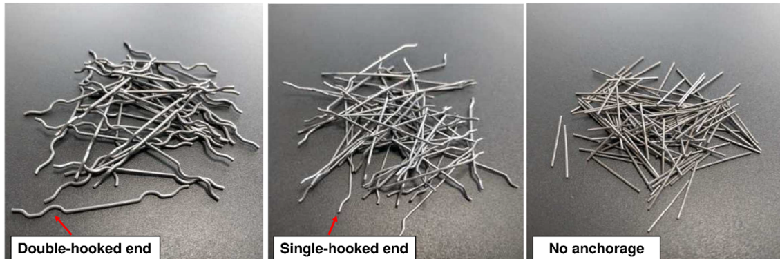
FIGURE 6 Steel fibres adopted for three-point bending tests. From left to right: READYMESH MX-500, READYMESH MS-350, and READYMESH MM-150
