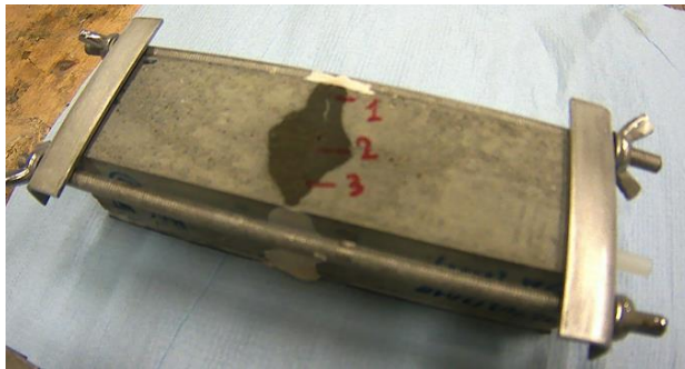
Fig. 4. Typical sample for which the crack width was controlled using the active crack width control technique. In the figure it is possible to see the healing agent released from the ruptured capsule and spread around the crack mouth (dark colored zone)
