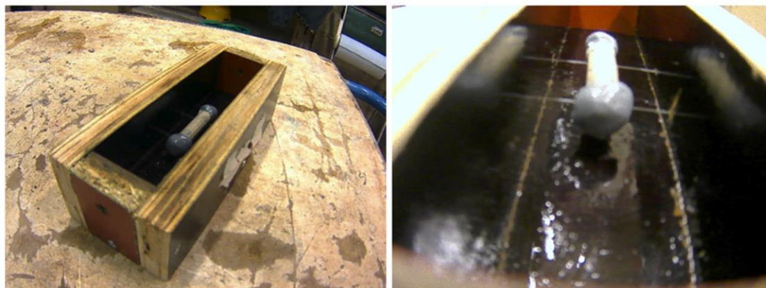
Fig. 2. Cementitious capsule fixed at its position at the bottom of the molds with nylon threads before the positioning of the oiled bar and casting (cross section in Fig. 3).
