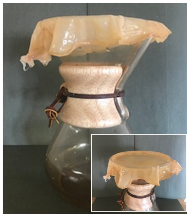
Figure 3. Point of use application with potential operational setup for gravity LFM filtration. Inset shows top of filter supporting feedwater.
