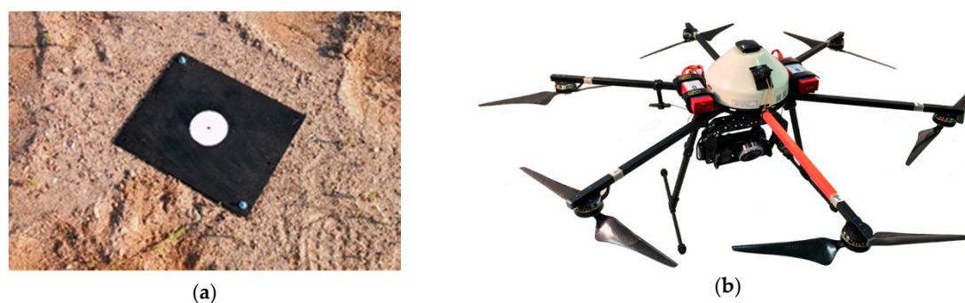
Figure 2. The equipment operated by the Laboratory of Geomatics of the University of Pavia: (a) an example of the used artificial markers and (b) the HEXA-PRO Unmanned aerial vehicle (UAV) used for the survey.
