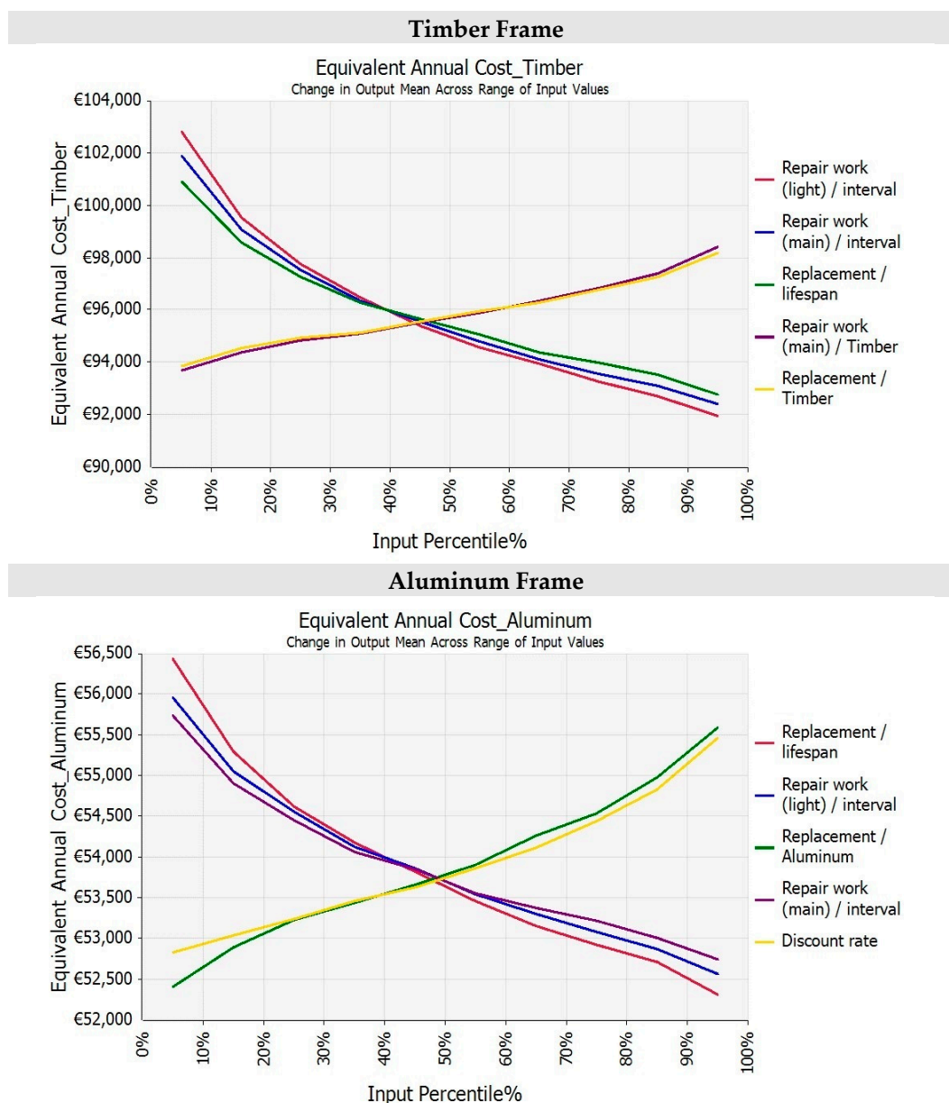
Figure 8. Spider graphs, Timber/Aluminum frames, for stochastic Equivalent Annual Cost. MCM simulation output.
