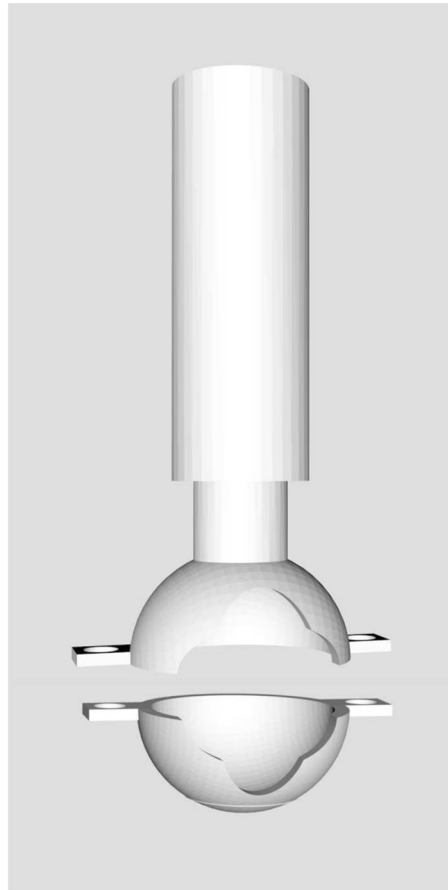
Figure 2. A computer-aided design of the retrofit attachment, dedicated to the Novint Falcon. The two parts are joined together to encapsulate the spherical end-effector. The circular cutouts necessitate rotation of the attachment around the end-effector, prompting movement of the wrist.
