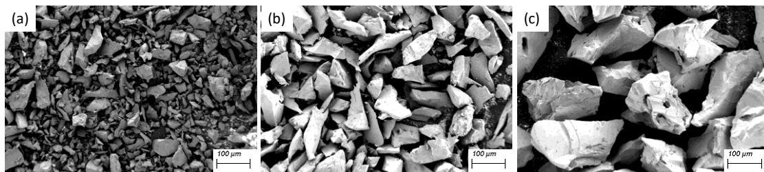
Figure 2. SEM micrographs of the three different sizes of sharp-edged alumina particles: (a) 60 \mu\text{m} , (b) 90 \mu\text{m} , and (c) 200 \mu\text{m} .
