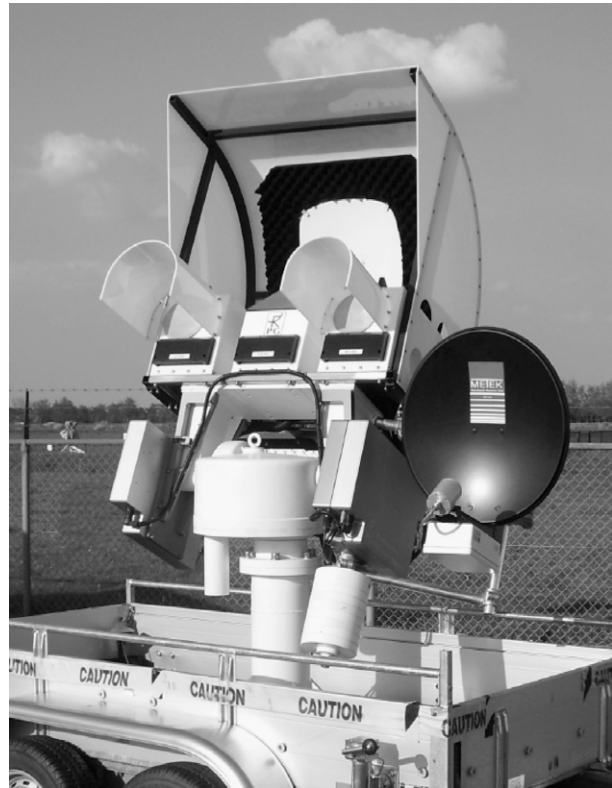
FIG. 1. The ADMIRARI radiometer at the Cabauw Experimental Site for Atmospheric Research (CESAR) observatory. On the right side (black antenna) a micro rain radar system is installed.
