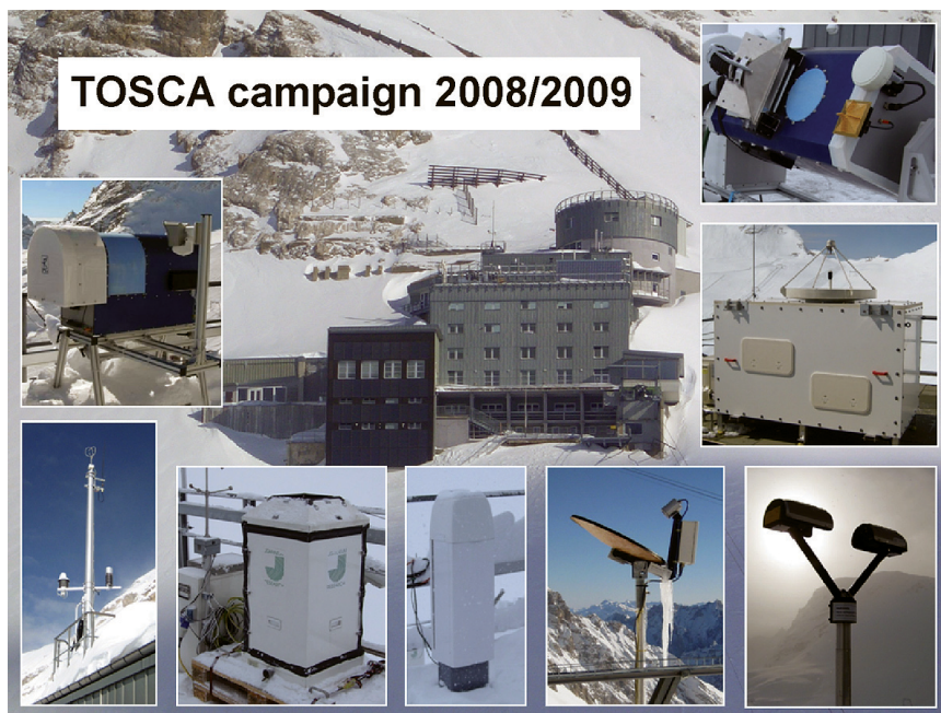
FIG. 1. Impressions of instruments deployed at (middle) UFS located at the mountain of Zugspitze in the German Alps during the TOSCA measurement campaign in the winter season 2008/09: (middle left) microwave profiler HATPRO; (bottom left)–(bottom right) 10-m meteorological mast, 2DVD, ceilometer, MRR, Parsivel disdrometer; (middle right) 36-GHz cloud radar MIRA36; (top right) 90-/150-GHz radiometer DPR.
