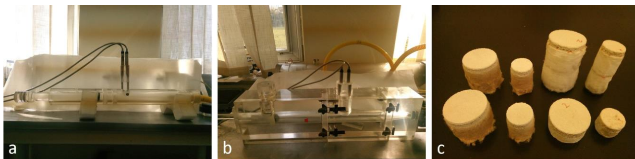
205 Fig. 2. Measurements set-up in the impedance tube with a diameter of a) 30 mm and b) 50 mm, and 206 c) circular samples of the four materials with a diameter of 30 and 50 mm.
