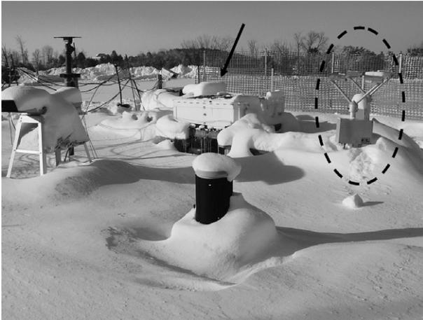
FIG. 1. Picture of the CARE site located 80 km north of Toronto at 44.23°N, 79.78°W at a height of 249 m MSL. The 2-DVD (pinpointed by the arrow) and the two PARSIVEL disdrometers (within the dashed ellipse) are visible in the center and on the right side (private picture taken by Peter Rodriguez, Environment Canada).
