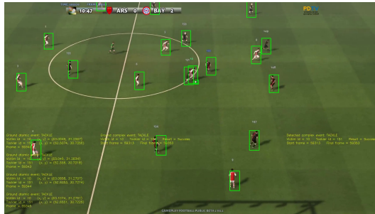
Fig. 1: Example of scene generated by the Gameplay Football engine, with superimposed ground truth bounding boxes and IDs of each player and the ball. The ground truth and detected events are also overlaid on the bottom of the scene: in this frame, a tackle attempt is correctly detected.
