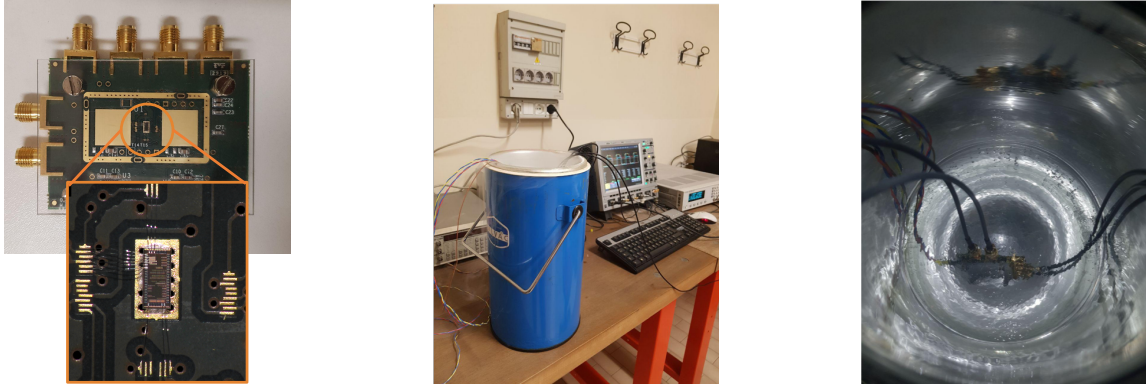
Figure 7. From left: The Test Chip is wire bonded in the center of the test board; Test setup used to measure time delays; Test board is dipped inside the small dewar in a bath of liquid Nitrogen at 77 K.
