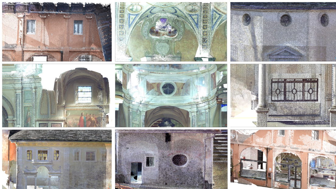
Figure 9. Different typologies of windows and doors. For the latter, their opening has sometimes affected the points acquisition.
