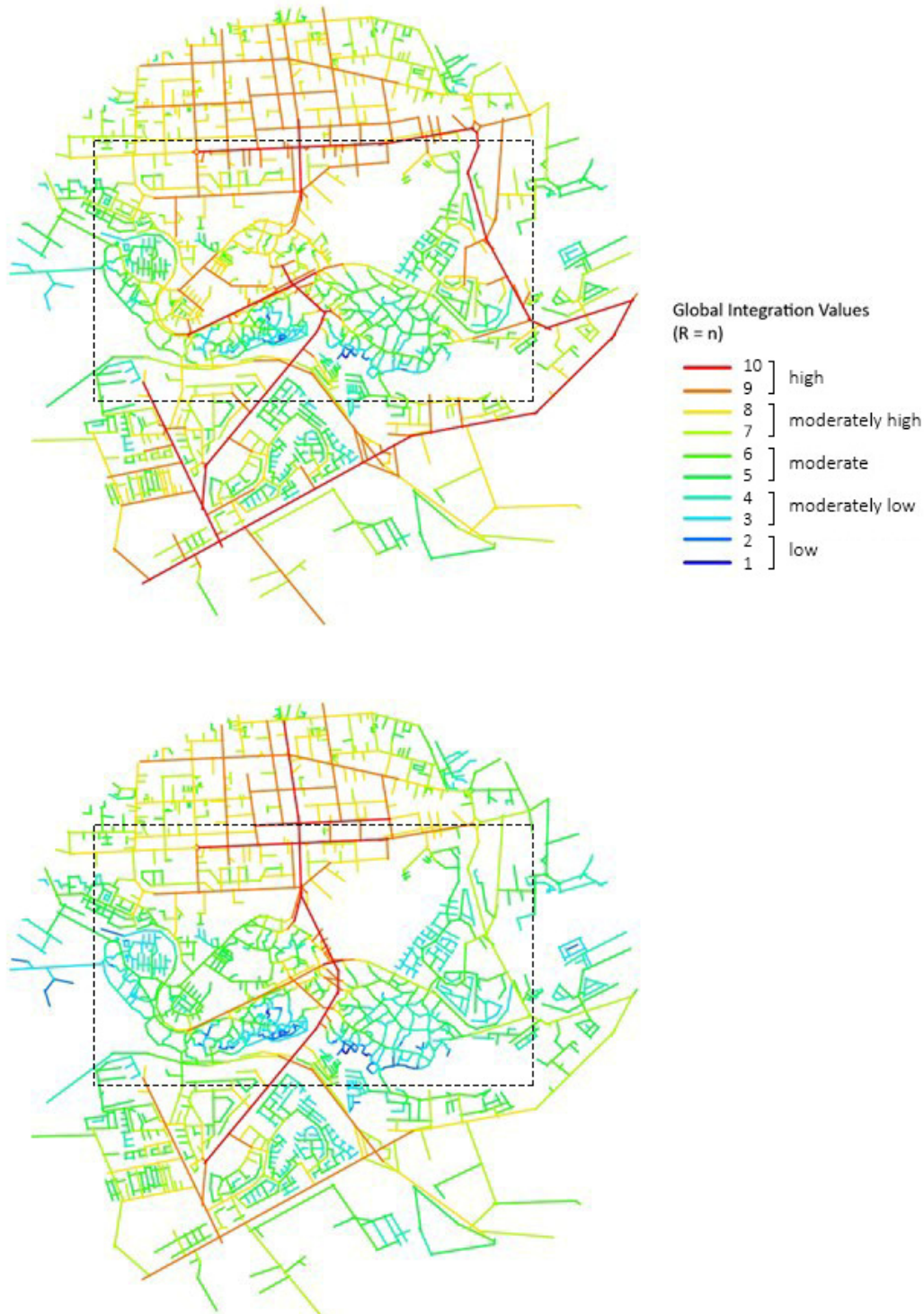
Figure 3. Axial maps of the current (top) and the future (bottom) configuration of Kibera public spaces (Elaborated by the authors).
