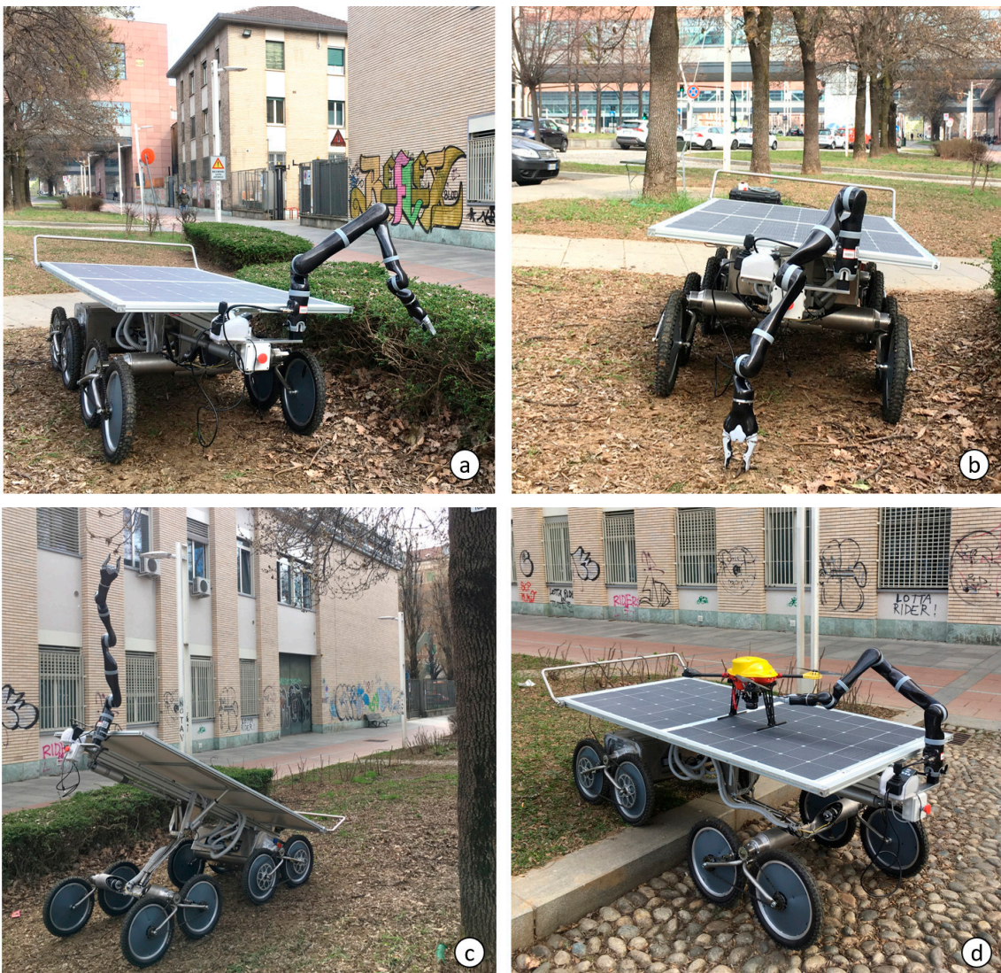
Figure 14. Agri.q02 in different configurations. (a) The robotic arm works on the rover side; (b) the arm reaches the soil; (c) the arm grasp a sample at the maximum height, with the rover pitch angle activated; (d) Agri.q02 compensate the slope and the step by using pitch and roll angle, to keep the landing platform horizontal.
