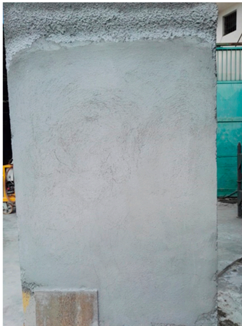
Figure 6. Pouring plaster results after two days from its application on the panel.
