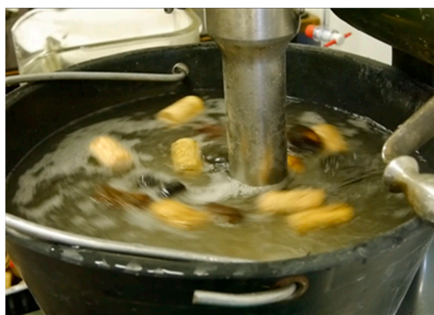
Figure 5. The bath extractor separator as a product of separation with stoppers (cork and synthetic).
