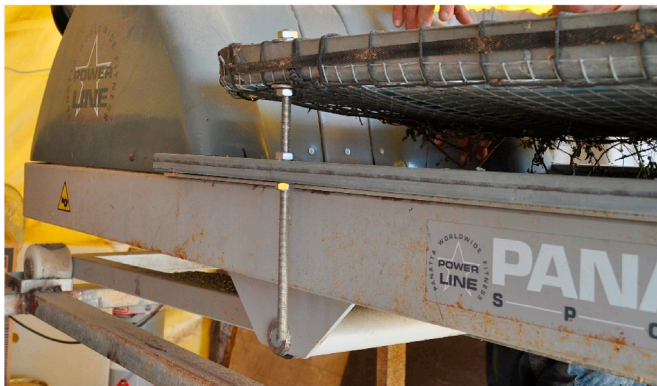
Fig. 6. Machine for detaching the dried leaves of the oregano plant.
