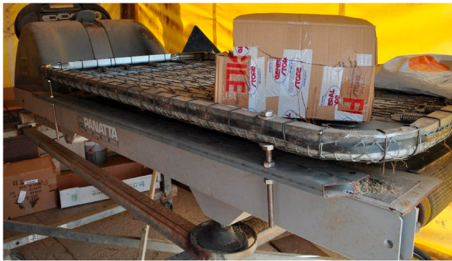
Fig. 5. Self-produced chestnut deburring machine.
