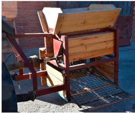
Fig. 5. Self-produced chestnut deburring machine.
