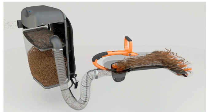
Fig. 11. Backpack combine harvester functioning.
