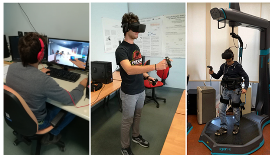
Figure 1: VR environments considered in this study: desktop VR (DVR, left), immersive VR (IC, center) and treadmill based immersive VR (KAT, right).
