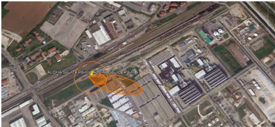
Figure 1. Possible toxic releases of acrylonitrile or benzene due to a hole of 3 cm in the rail tanker, following a seismic event. The release can interest residential areas along the railway.
