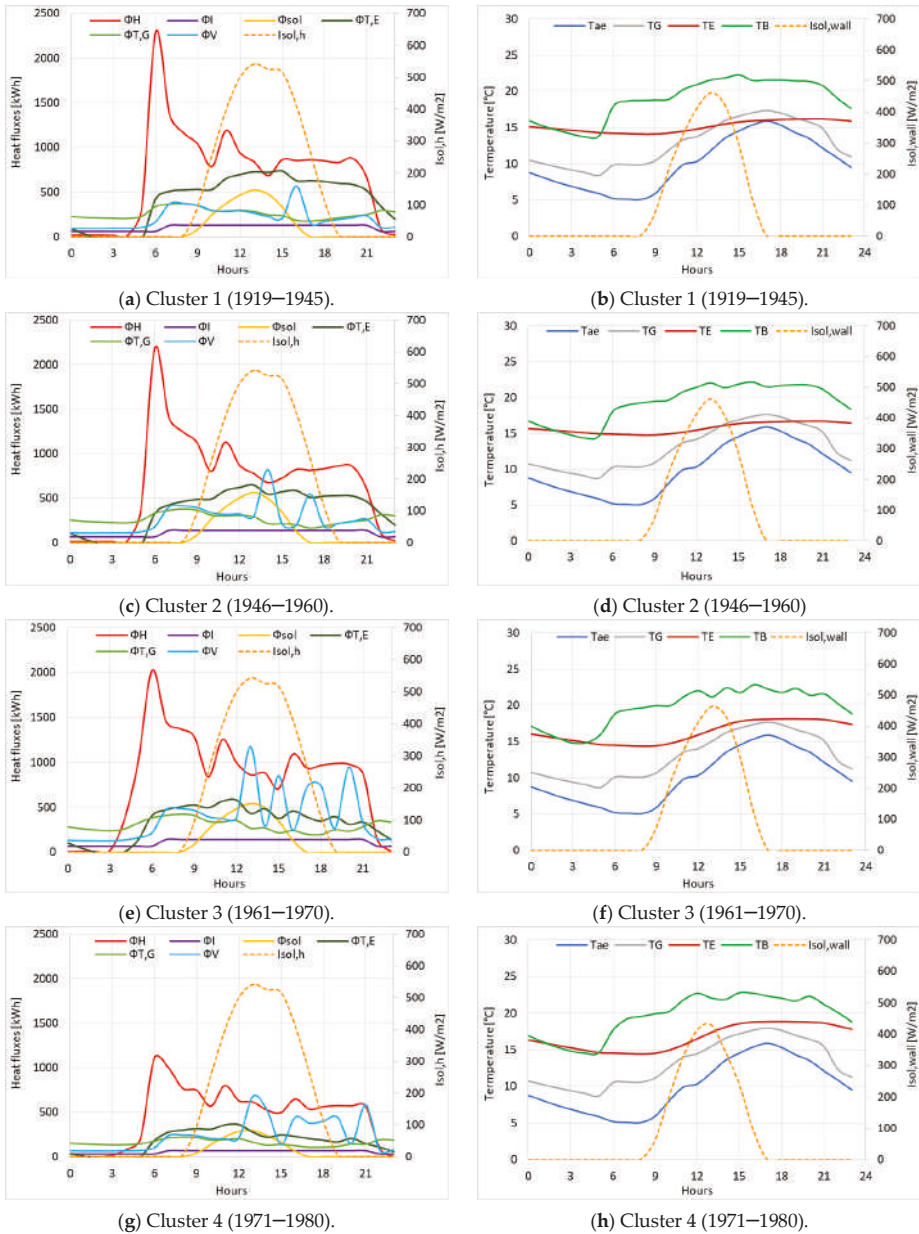
Figure 8. Heat flux components and building temperatures (with a variable number of air changes per hour and windows opening) for a typical day: February 22nd 2014, with a T_{ae} = 6.24 °C (clusters for the four construction periods).
