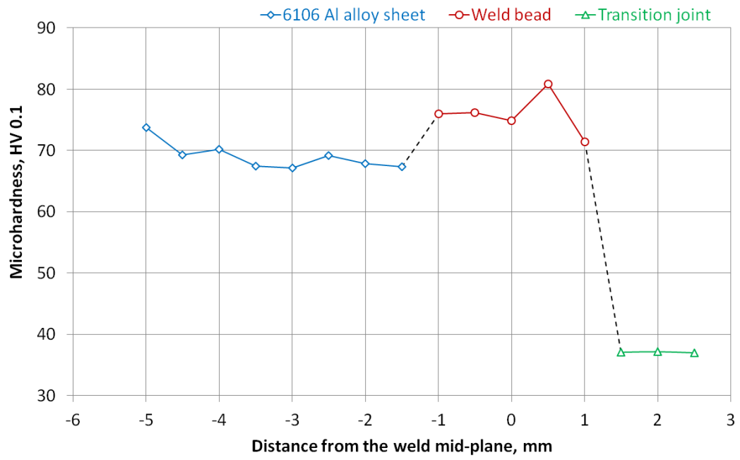
Fig. 11: Microhardness of the weld between the 6106 Al alloy sheet and the transition joint. Type C hybrid joint.
