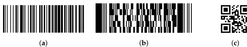
Figure 1. Barcode technology evolution: (a) code 128, (b) code PDF417 and (c) quick response (QR) code.
