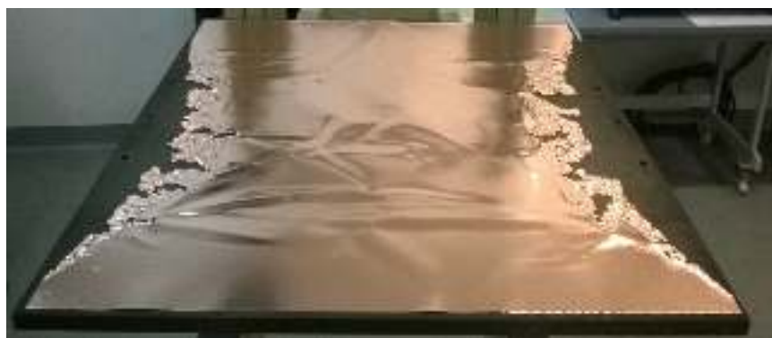
Figure V.6. Higher T near the edges of the substrate causes local Cu melting while the inner part is unaffected.
