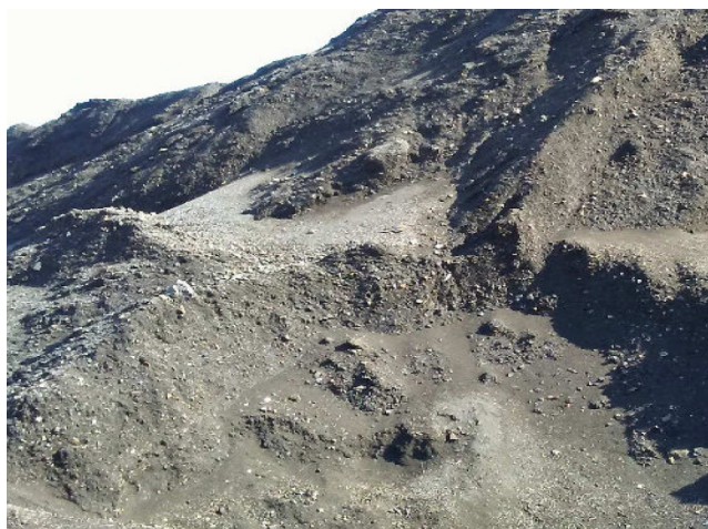
Fig. 1. Granular material arising from comminution and sieving of mix of soils, glass, gypsum, rockwool, glasswool (image at 10m scale).
