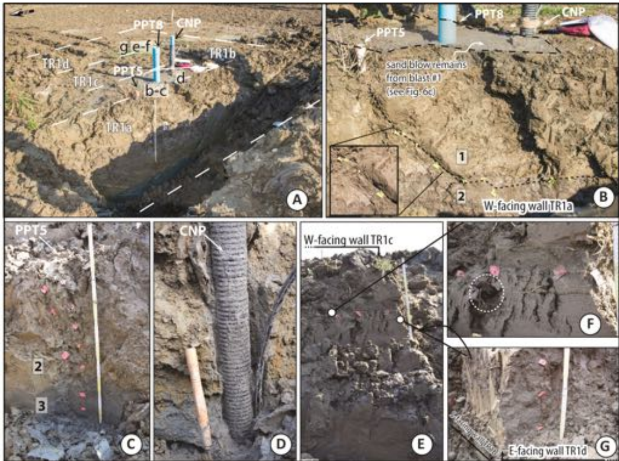
649 650 Fig. 13. Geometrical arrangement of the trenches (a); details of the most significant features 651 exposed in the walls. Sand boils from the blast test (b) were generated by sand moving upward 652 using the PPT5 pore pressure transducer, colored flags in (c), and the external part of the CNP 653 profilometer (d) as conduits. Sand from CNP moved sub-horizontally, as shown by yellow flags, in 654 (b). The white dashed circle in (f) indicates the remnants of the vegetation at the ground surface, 655 covered by the 2012 sand blow (bottom of the blow marked by colored flags in e, f). Details of the 656 2012 vertical path (colored flags) developed along a thin fracture in (g).
