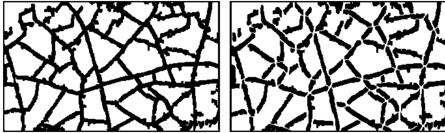
Fig. 3. Panel A in Figure 2 as pre-processed for the analyses of the crack orientation. Edges are enhanced by means of the Dilate GIMP filter (left panel) and then separated by removing the crossing points (right panel).
