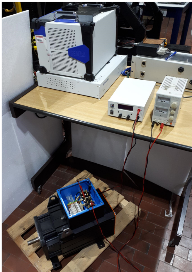
Fig. 10. Experimental setup: dual winding machine, DC power supplies and HBM Gen7i data logger.
