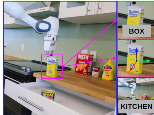
Fig. 1. The ability of a robot to perform multiple tasks at the same time is crucial. For example, to manipulate correctly the object in the scene above, a robot should understand the class of the object, its orientation and the overall context where it operates. Image courtesy of NVIDIA Robotics Research Lab, Seattle ( news.developer.nvidia.com/nvidia-opens-robotics-research-lab-in-seattle/ ).
