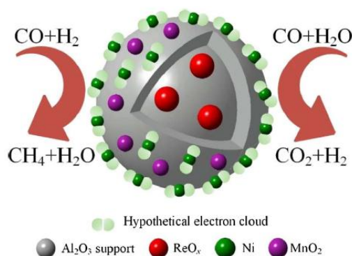
Scheme 2. Scheme of the processes occurring at the surface of Re-promoted Ni-Mn bimetallic particles on Al 2 O 3 support. Reprinted from Appl. Catal. A Gen. , 552, Dong, X.; Jin, B.; Sun, Y.; Shi, K.; Yu, L., Re-Promoted Ni-Mn Bifunctional Catalysts Prepared by Microwave Heating for Partial Methanation Coupling with Water Gas Shift under Low H 2 /CO Conditions. Copyright (2018) with permission from Elsevier.
