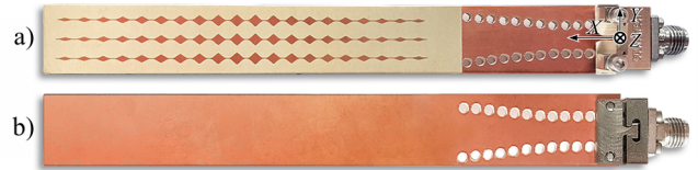
Fig. 5. Fabricated LWA using Rogers RT6010 with a rated relative dielectric constant \epsilon_r = 10.2 , thickness h = 1.27 mm: (a) top view (b) bottom view.
