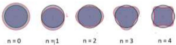
Fig. 6. Bore distortion orders.
