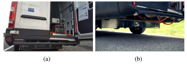
Fig. 4: Receiver structure mounted under the vehicle. Rear view (a), with the PE in the red box inside the vehicle. Detailed view (b).
