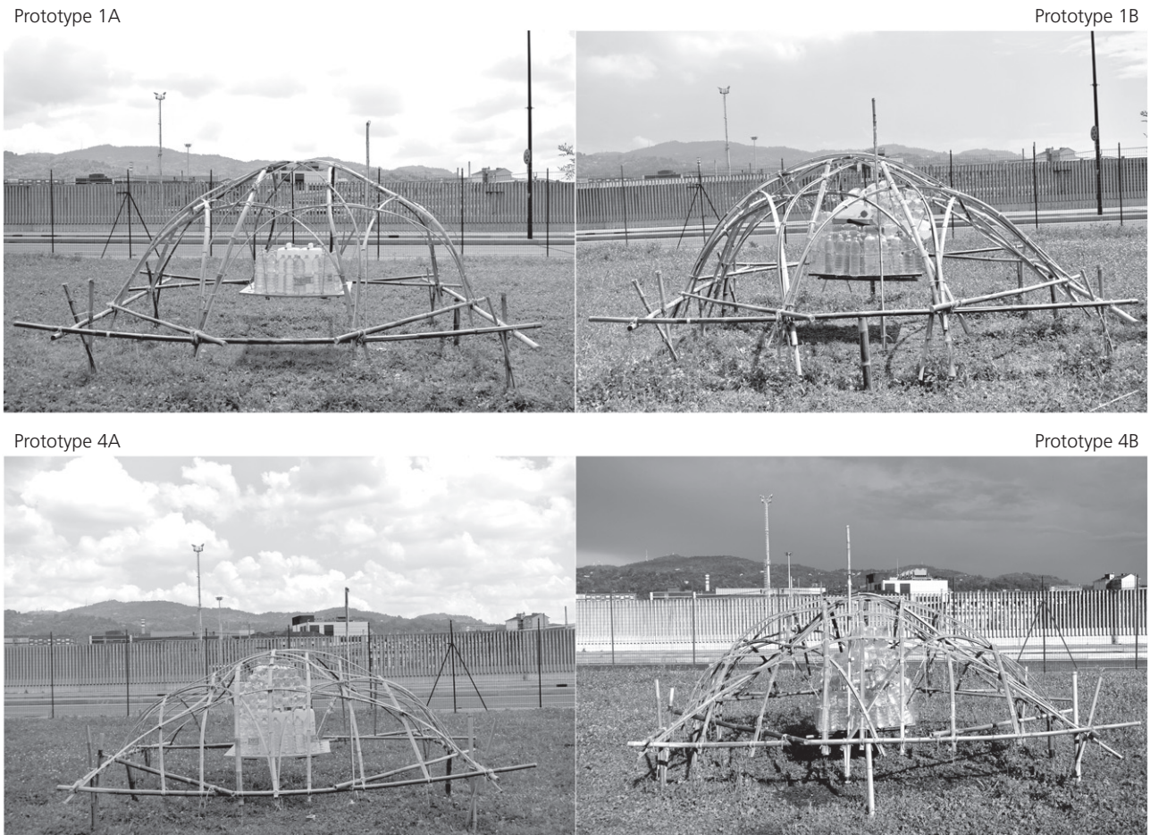
Figure 7. Comparison of loading and deformations in prototypes 1A and 4A to their respective 'enhanced' versions, 1B and 4B
