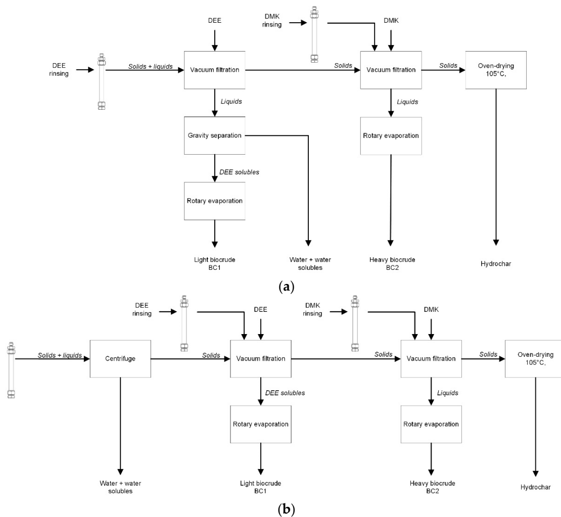
Figure 1. Scheme of Procedure 1 (a) and 2 (b) for products collection.
