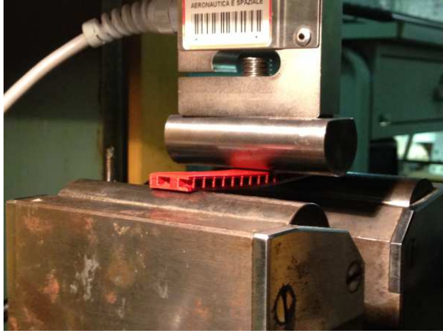
Figure 2: Specimen 1 during the three-point bending test.
