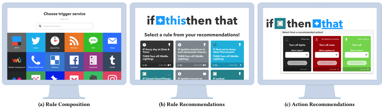
Figure 1: TAPrec is an EUD platform that supports the composition of trigger-action rules with dynamic recommendations. Users can compose IF-THEN rules in an IFTTT-like web application (a). By analyzing the rules saved by the users, TAPrec is able to recommend new rules to be used (b) and actions for auto-completing a the rule that is being composed (c).
