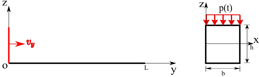
Figure 18: A metallic beam under the moving load.
