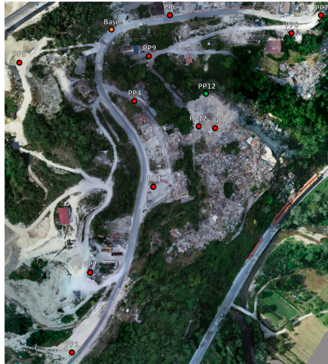
Figure 9. Locations of the 12 GCPs in Pescara Del Tronto used in the 2018 Optimized model (red represent surveyed fabricated GCP markers, green indicate natural GCP markers, and orange is the base station location).
