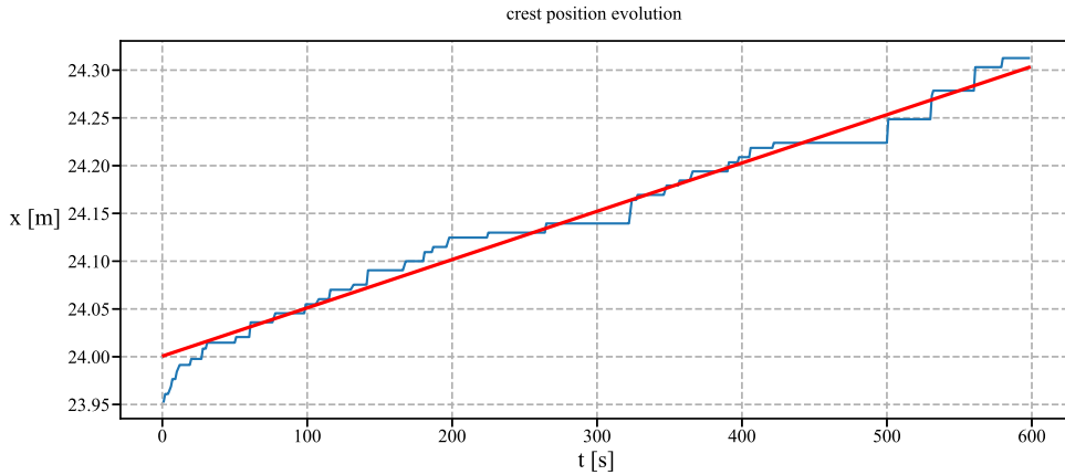
Fig. 8. Mean crest position highlighting a nearly constant migration speed after an initial transient of about 20 s.
